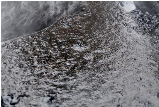
Figure 2: Low fuming polymer layer development and margin beyond which asphalt fumes are still visible.
