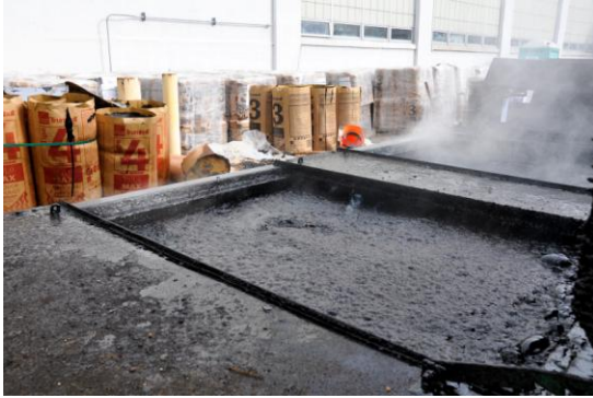
Figure 1: Large kettle at uniform temperature with low fuming layer in foreground and no layer in background.
