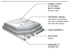
THERMAPINK<sup>®</sup> extruded polystyrene (XPS) insulation, installed entirely above the roof deck and continuous, is shown in Figure 2.
