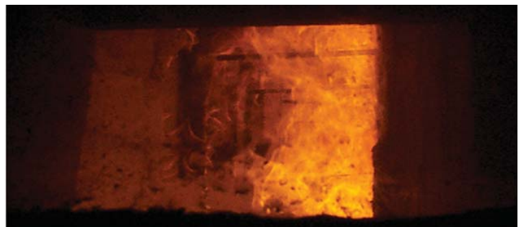
Fire Exposure Inside ASTM E119 Furnace
