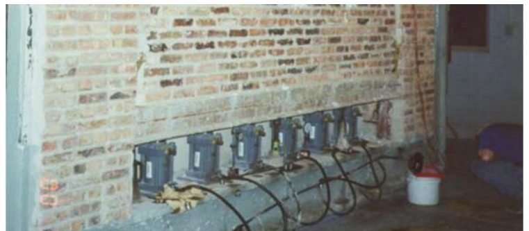
ASTM E119 Test Assembly, Exterior Side
