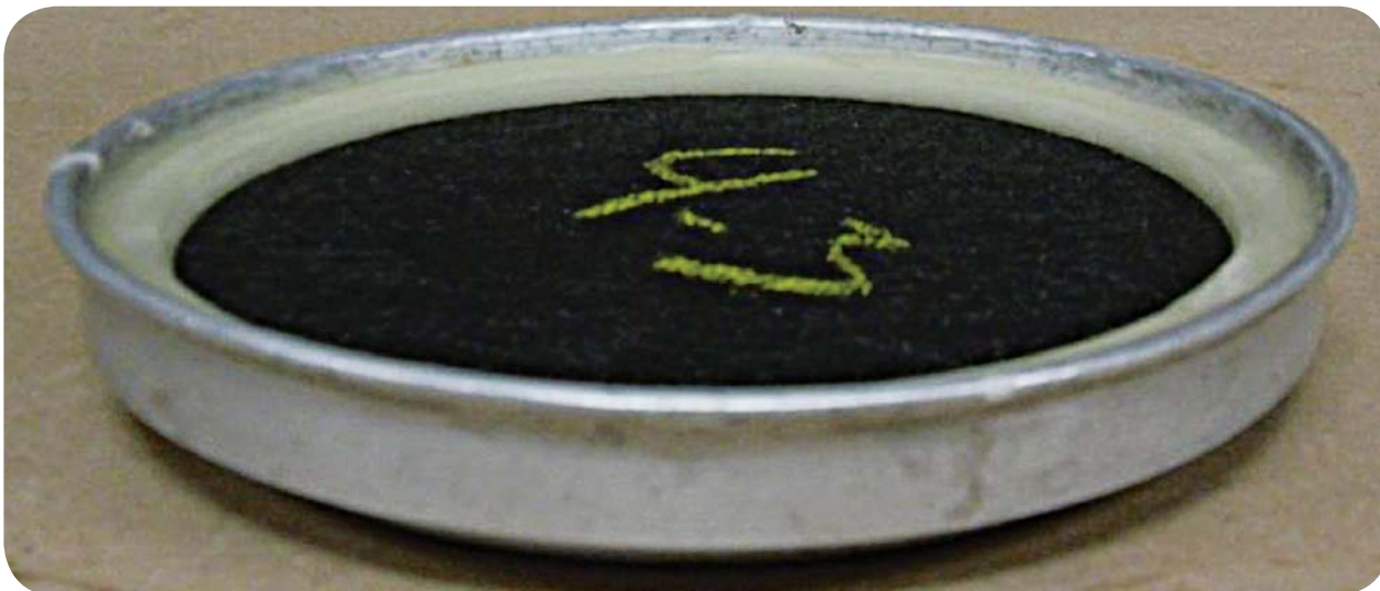
Figure 2: #15 Felt Underlayment Sample–ASTM E 96–6" dia. “Dry Cup”
