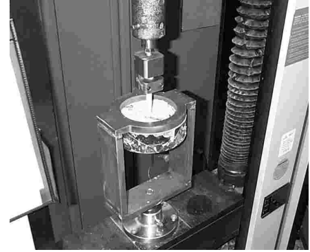
Figure 3 – A test setup for pullout testing.
