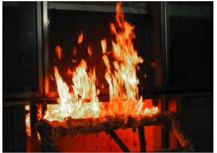
ASTM E2307 room and exterior window burner fire exposure.
