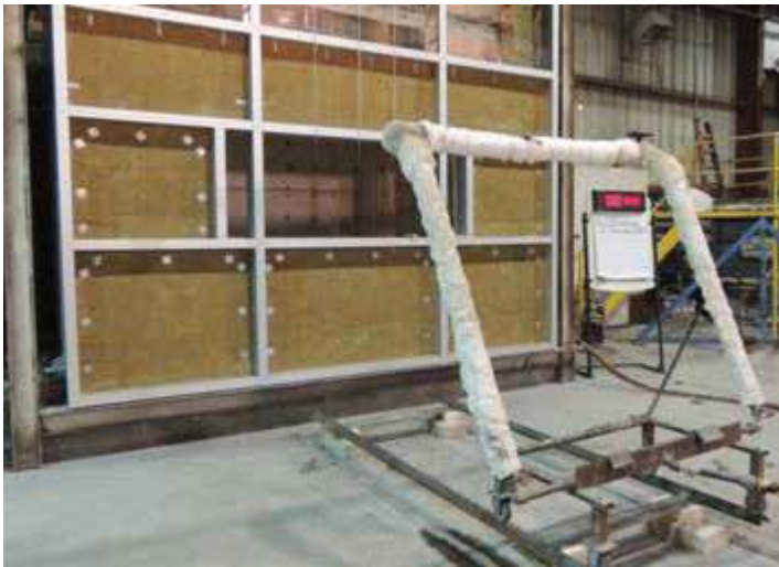
ASTM E2307 intermediate scale, multi-story, test furnace, and the test wall frame used to hold the test wall and perimeter fire containment systems.
