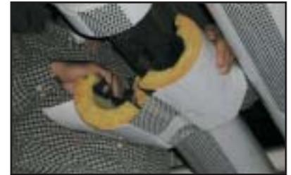
*A VaporWick insulation sample is removed for testing after three years in service.*
