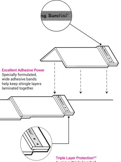
A unique "triple layer" of reinforcement occurs when the fabric overlays the common bond of the laminated layers, offering excellent fastener holding power.
