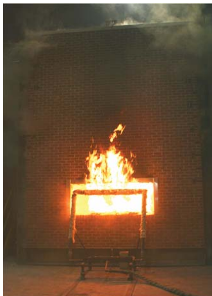
Fire emitting from the NFPA 285 test window.
