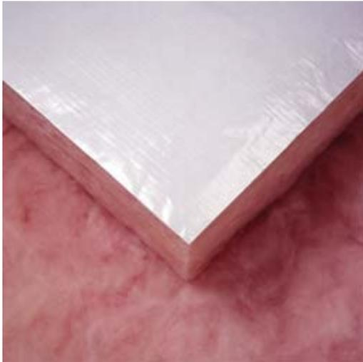
EcoTouch® Flame Spread 25 FIBERGLAS™ Insulation with PureFiber® Technology is a light density, flexible batt, with a factory applied facing that has an assured low flame spread. The product is available in R-values ranging from 11 to 30. The FSK (foil-scrim-kraft) and light reflective white PSK (polypropylene-scrim-kraft) facings act as vapor retarders, and provide a neat, finished appearance.
