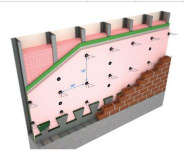
The CavityComplete® Wall System excludes the masonry veneer, steel studs and interior and exterior gypsum board. A detailed list of the components is available at www.CavityComplete.com.
