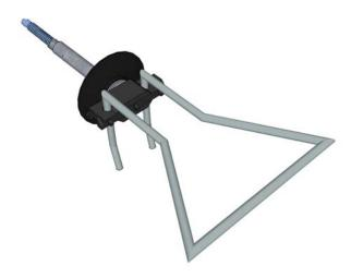
Barrel screws are available in 9 lengths (5/8", 1", 1-1/2", 2", 2-1/2", 3", 3-1/2", 4" and 4-1/2"). Barrel screws penetrate both the rigid insulation and the gypsum board before making contact with the backup. Barrel screw length is determined by a combination of the thickness of the FOAMULAR® Extruded Polystyrene (XPS) and the exterior gypsum board sheathing. For example, 2" continuous insulation over 5/8" exterior gypsum sheathing requires a 2-1/2" long barrel screw.
