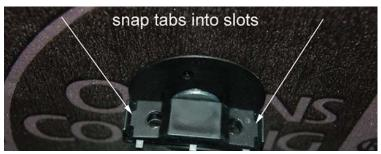
Make sure tabs snap into the sides using needle nosed pliers if necessary to ensure closure
