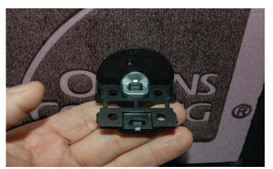
Place tab in Pos-I-Tie® barrel slot
