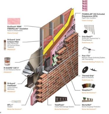
The CavityComplete® Wall System excludes the masonry veneer, steel studs and interior and e gypsum board. A detailed list of the components is available at www.CavityComplete.com
