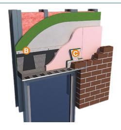
The Cavity Complete® Wall System excludes the masonry veneer, steel studs and interior and exterior gypsum board. A detailed list of the components is available at www.CavityComplete.com
