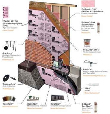
The CavityComplete® Wood Stud Wall System excludes the masonry veneer, wood studs, interior gypsum board and exterior sheathing. A detailed list of the components is available at <a href="www.CavityComplete.com">www.CavityComplete.com</a>.
