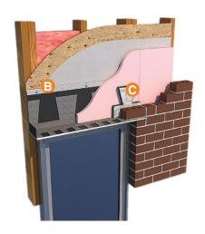
The CavityComplete\* Wood Stud Wall System excludes the masonry veneer, wood studs, interior gypsum board and exterior sheathing. A detailed list of the components is available at <a href="https://www.CavityComplete.com">www.CavityComplete.com</a>.
