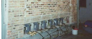
ASTM E119 Test Assembly, Exterior Side
