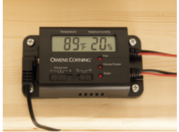
Attic-Mounted Controller Module
