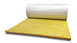
Fiberglas™ FLEXWRAP® is a flexible insulation product made from fiberglass blanket bonded together with a thermosetting resin. The fibers are oriented to provide good compressive strength while providing flexibility during installation. FLEXWRAP® insulation is suitable for operating temperatures up to 850°F (454°C). Available in ASJ or FRK facings.
