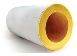
Owens Corning® Large Diameter Fiberglas™ Pipe Insulation is molded of heavy density resin bonded inorganic glass fibers that come in one-piece, 36" (914mm) long, hinged sections. Sections begin at 18" O.D. through 42" O.D. and can be ordered as factory applied SSL® with ASJ Max or as unjacketed No-Wrap.
