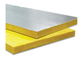
Types 703 and 705 Series Insulation Boards are made of inorganic glass fibers with a thermosetting resin binder and formed into semirigid or rigid rectangular boards.
