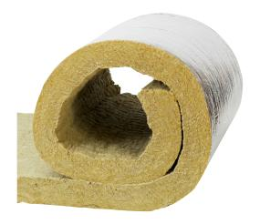
Thermafiber® Industrial Wrap, made with Paroc® technology, is a mineral wool wrap capable of withstanding high temperatures and is designed to be used in industrial equipment and applications. This product is used to insulate large diameter piping, vessels and ducts. Thermafiber® Industrial Wrap is available with or without a reinforced alulaminate facing.
