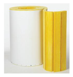
Fiberglas™ Pipe and Tank Insulation is made of semi-rigid fibrous glass board material, factory-jacketed with an FRK or ASJ Max jacket. The insulation is adhered with the end grain perpendicular to the jacket. This provides a flexible product that is easily wrapped around pipes, tanks or irregularly shaped objects, while providing good rigidity and abuse resistance.
