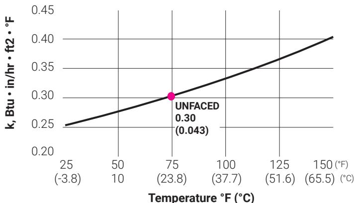
Apparent thermal conductivity curve determined in accordance with ASTM Practice C1045 with data obtained by ASTM Test Method C177. Values are nominal, subject to normal testing and manufacturing tolerances.
