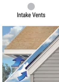
Help prevent heat and moisture buildup in the attic by allowing fresh air to enter the attic.
