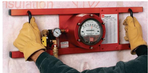
The Inspect-R® insulation density gauge is used to verify the R-value of Owens Corning® PROPINK Complete™ Fiberglas™ in a wall cavity.<sup>†</sup>
