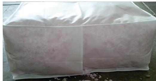
The Attic Hatch Bag is a loosefill insulation bag that can be used for the attic hatch, an insulation block at the eaves, or as fencing around the attic opening. The fabric bag is flexible to different hatch sizes. Simply fill the bag with 7 lbs (1/4 of a bag) of loosefill insulation to achieve R-60. The bag self-seals when you pull the hose out. (Bag in picture is shown filled.)
