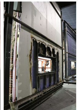
Figure 6: Interior of test wall following test showing no intrusion into upper level
