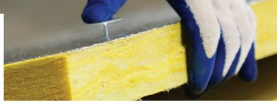
Types 703 and 705 Series Insulation Boards are made of inorganic glass fibers with a thermosetting resin binder and formed into semi-rigid or rigid rectangular boards. Types 703 and 705 are available with factory-applied FRK or poly-encapsulated ASJ Max facings. Both facings are vapor retarders and provide a neat, finished appearance in mechanical applications.
