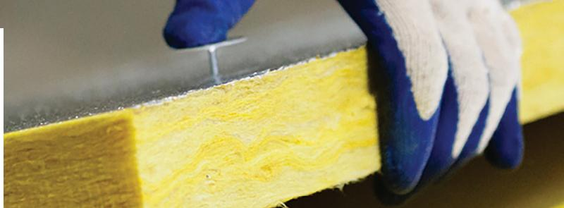
Types 703 and 705 Series Insulation Boards are made of inorganic glass fibers with a thermosetting resin binder and formed into semi-rigid or rigid rectangular boards. Types 703 and 705 are available unfaced and with factory applied FRK or poly encapsulated ASJ Max facings. Both facings are vapor retarders and provide a neat, finished appearance in mechanical applications.
