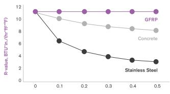
Tie connector penetration rate, % of the total area of the panel
