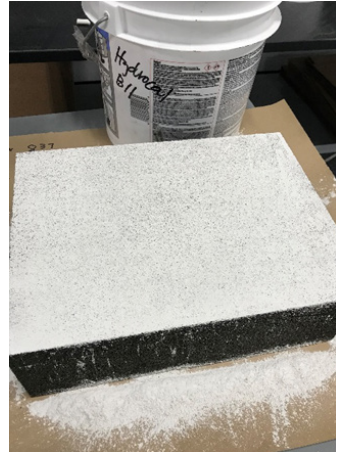
Step 4 Allow excess powder to fall off the edge of the block. (Save excess for next side.)
