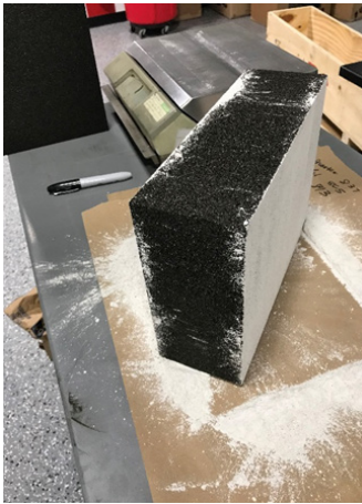
Step 5 Turn block over and repeat application, saving excess powder for the next block.
