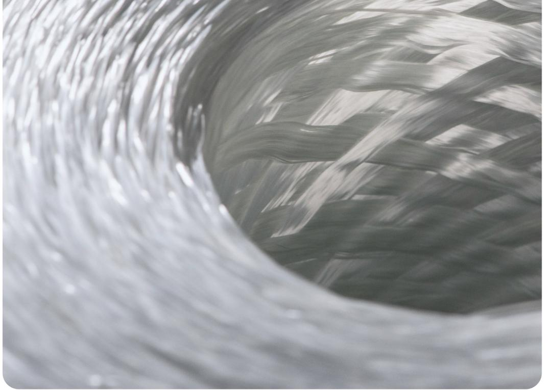
K247 multi-end spun roving is specifically designed to provide extra reinforcement in the transversal direction.
