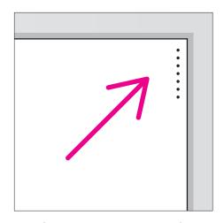
**Identify the installation direction** of the Bright &  $Up^{\mathsf{m}}$  overlay tile based upon the location of the holes.
