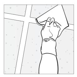
**Clean/degrease** the grids before renovation tile installation\*.
