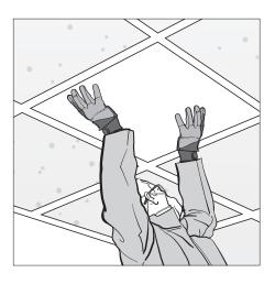
Lower ceiling tile and overlay onto the grid for a fresh new look
