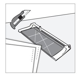
Cut the ceiling overlay with a cutter or a paper cutting machine for a cleaner cut. Up to two tiles can be cut at the same time.
