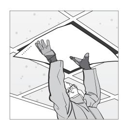
**Position** the Bright & Up<sup>™</sup> ceiling overlay tile, smooth side down, directly beneath the existing tile.
