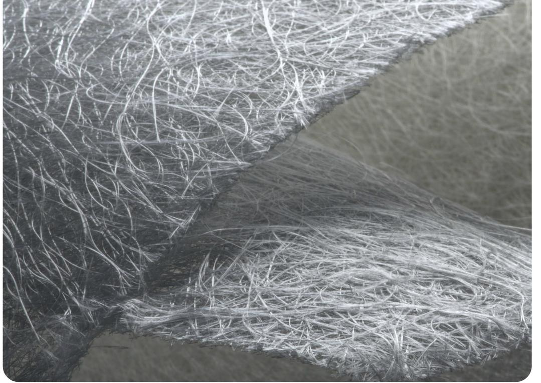
**M710B chopped strand mat represents a compelling solution where quick-wetting, rapid air release, good conformability, and low resin consumption are desired.**
