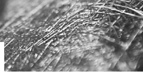
M710B chopped strand mat represents a compelling solution where quick-wetting, rapid air release, good conformability, and low resin consumption are desired.
