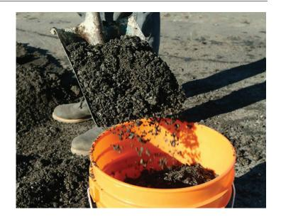
Reclaimed asphalt pavement (RAP) is created when old asphalt is milled into small pieces and added to a new mixture. RAP is used for a wide variety of applications, including highways, roads, airport runways, parking structures, and driveways.
