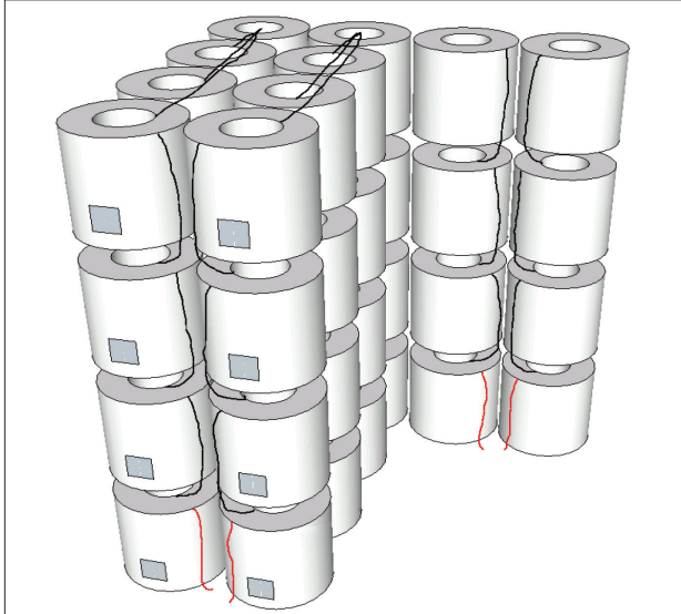
Creel-Pak® pallet spliced for 16 ends
