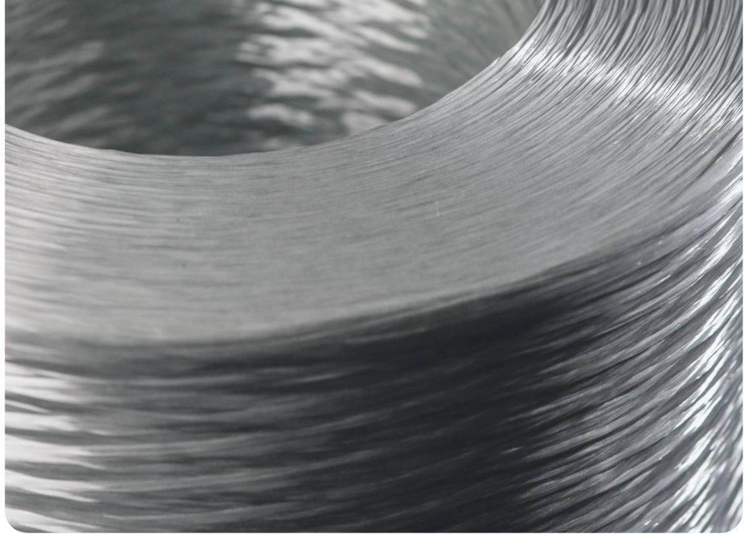
Ultrablade® 2 leverages the power of WindStrand® 4000's higher modulus at increased Fiber Volume Fractions to improve laminate modulus in the main fiber direction. Ultrablade® 2 allows more efficient blade design and enables the making of lighter, longer blades that reduce the cost of wind energy.
