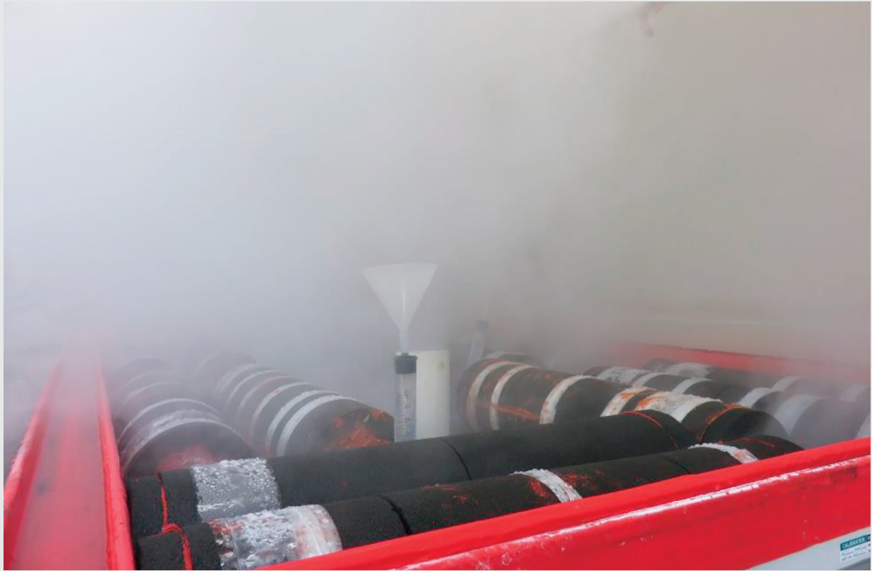
Figure 7 – Insulating systems were examined for the protection they provided against corrosive elements in a harsh environment.
