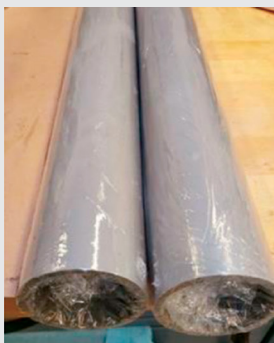
Figure 8 – Cellular glass insulation protected pipes from damage in a corrosive atmosphere; non-insulated pipes showed significant damage following the test's completion.
