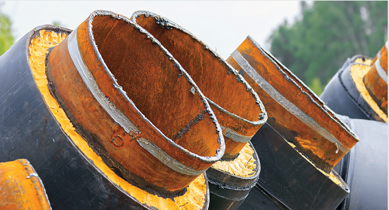
Figure 1 – CUI develops when moisture penetrates insulation or remains in contact with metal piping.
