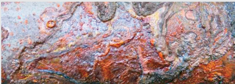
Figure 8 – Cellular glass insulation protected pipes from damage in a corrosive atmosphere; non-insulated pipes showed significant damage following the test's completion.
