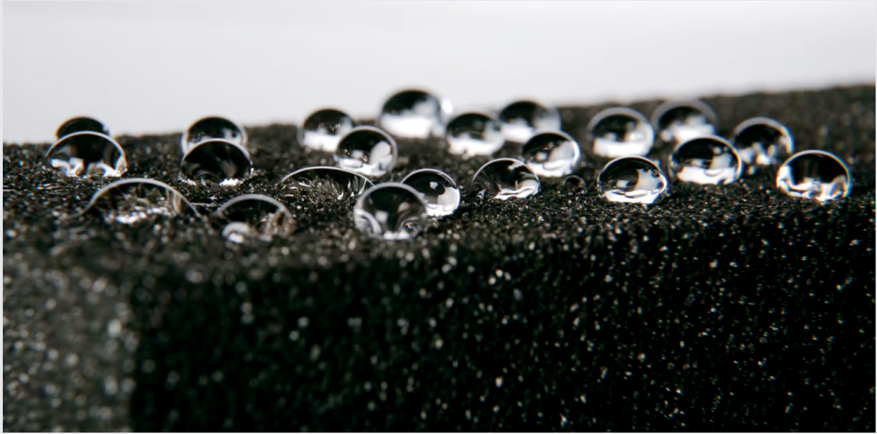
Figure 4 – Cellular glass insulation is made up of multiple closed-cell glass beads, making it impermeable and non-absorbent.
