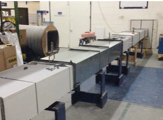
Figure 5 Picture of duct liner test setup per ASTM E477.
