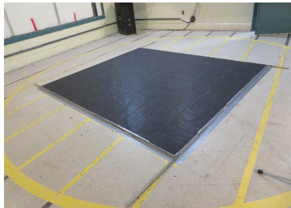
Figure 1a and 1b: Pictures of a sample duct liner being tested in reverberation chamber per ASTM C423.
