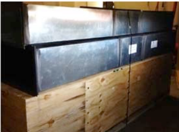
Figure 4 Picture of ten-foot-long test ducts prepared for ASTM E477 testing.
