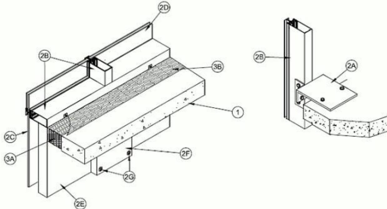
**1. Floor Assembly** — Min 4-1/2 in. (114 mm) thick reinforced lightweight or normal weight (100-150 pcf or 1600-2400 kg/m<sup>3</sup>) structural concrete.
