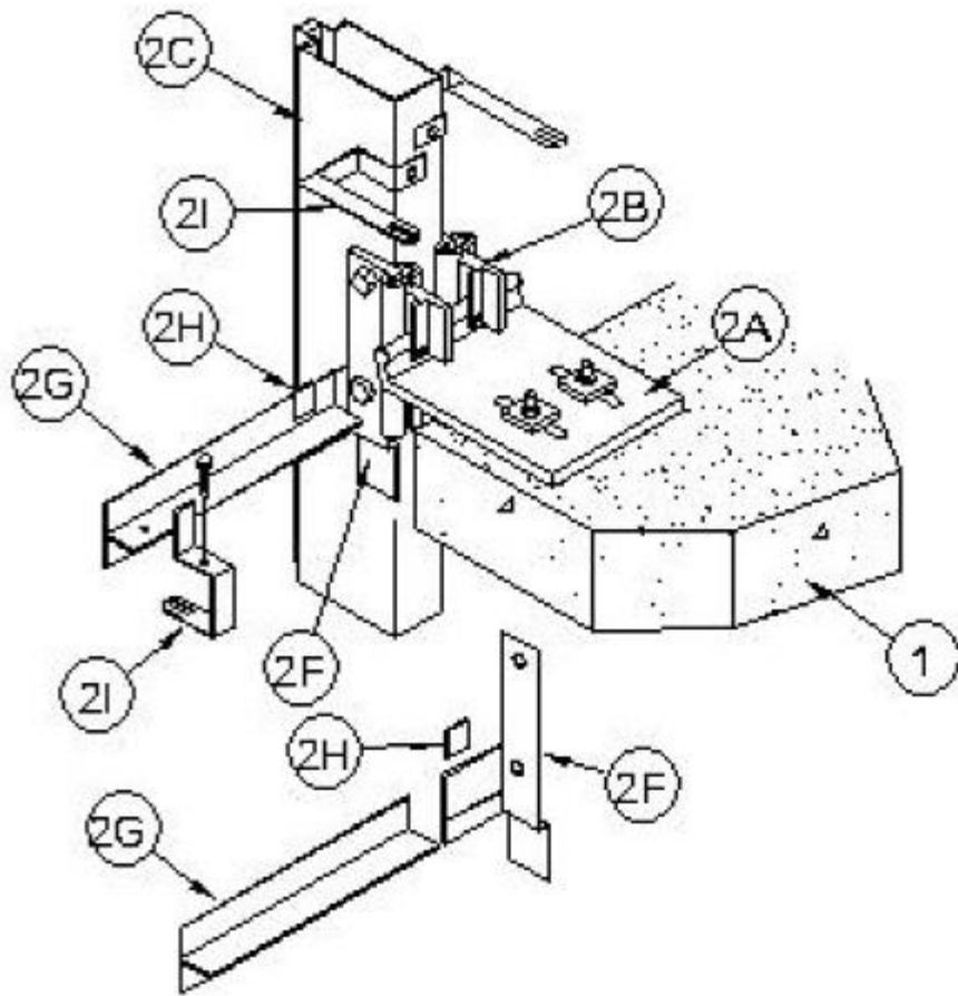
**1. Floor Assembly** — Min 4-1/2 in. (114 mm) thick reinforced lightweight or normal weight (100-150 pcf or 1600-2400 kg/m<sup>3</sup>) ) structural concrete.
