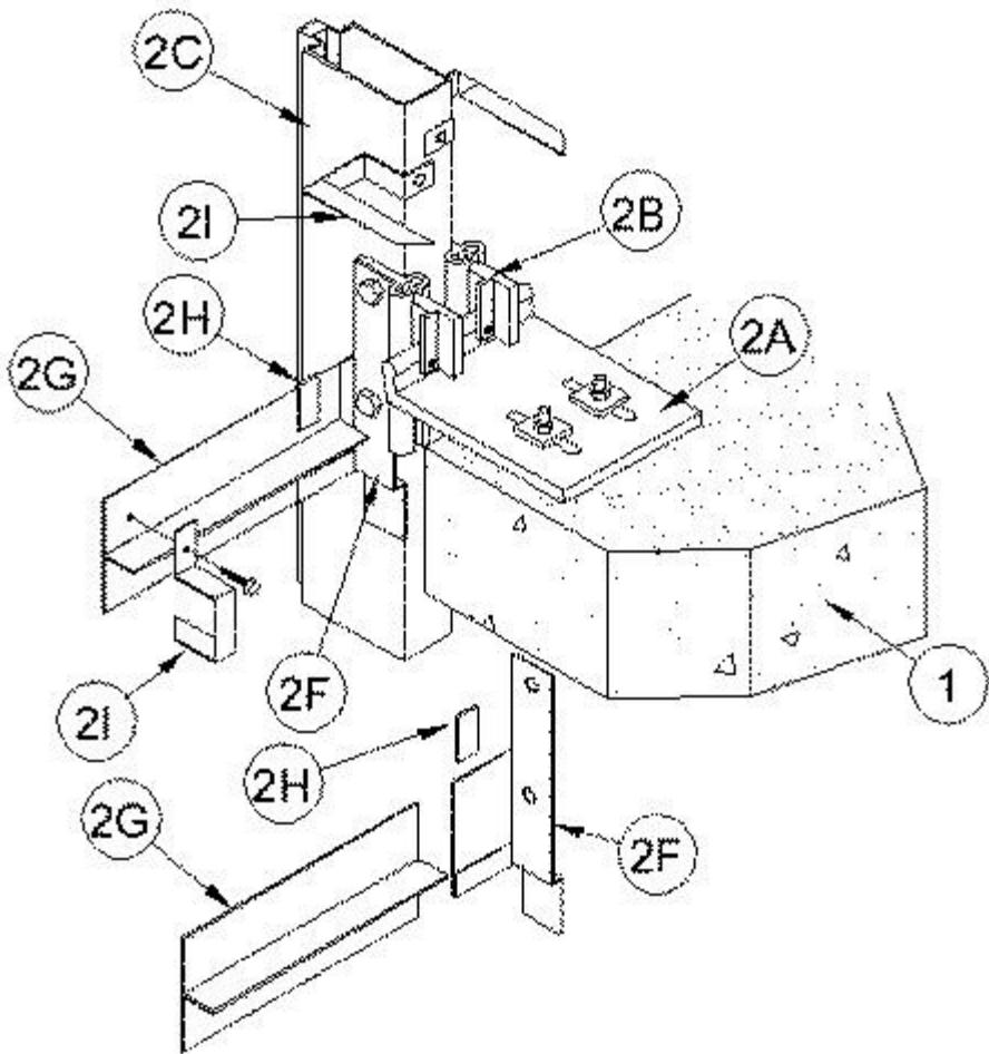
**1. Floor Assembly** — Min 6 in. thick reinforced lightweight or normal weight (100-150 pcf) structural concrete.
