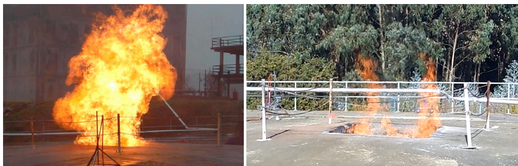
Figure 3. Flame height comparison: basin with and without FOAMGLAS® PFS™ Pool Fire Suppressant System Generation 2. 2
