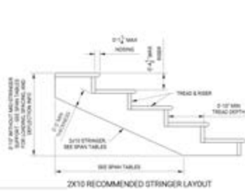
FIGURE 11: 2X10 RECOMMENDED STRINGER LAYOUT
