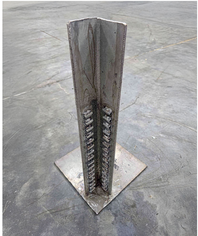
Figure 4. Thermocouple tree: before installation
