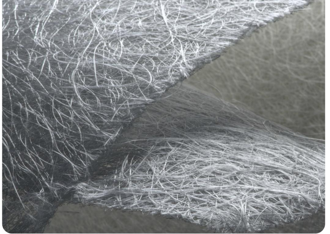
**M723A chopped strand mat represents an ideal solution for demanding applications requiring good surface finish and exceptional mechanical properties, in hand lay-up or closed mold processes.**
