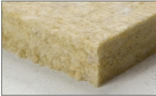
**Thermafiber® SAFB™** (Sound Attenuation Fire Blankets) are mineral wool insulation batts designed to provide acoustical control and fire protection in many UL® fire-rated wall and floor-ceiling assemblies. SAFB™ resists temperatures over 1,093°C (2,000°F) and can add points to STC for walls and floor-ceiling assemblies. SAFB™ can be installed in both steel stud and wood-framed construction.
