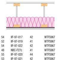
not less than 38 mm x 89 mm (1-1/2" x 3-1/2"), spacing and depth as specified below, 15.5 mm (5/8") OSB subfloor, resilient channels spacing specified below, single layer 15.9 mm (5/8") type "x" gypsum board ceiling finish; 152 mm (6") thickness QUIETZONE® PINK NEXT GEN® FIBERGI AS® Acoustic Batt Insulation
