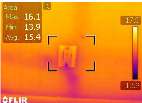
Figure 8: Minimal thermal penetration observed from framing surrounding an electrical fixture. Source: SAIT
