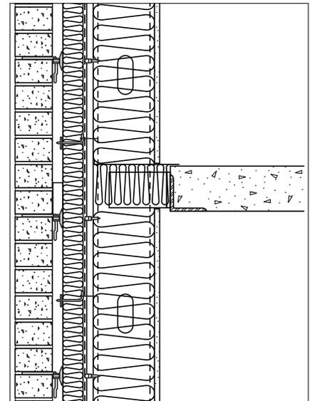
In today's designed assemblies with the emphasis on energy reduction and sustainable construction, we now see systems that incorporate air, water, and thermal efficiency all in one assembly. These systems must work correctly and in concert with each other in order for the entire wall assembly to perform as desired.
