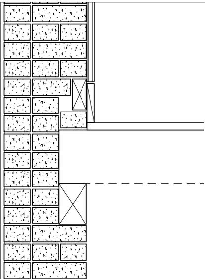
In the 1900s, an exterior wall would have no insulation.
