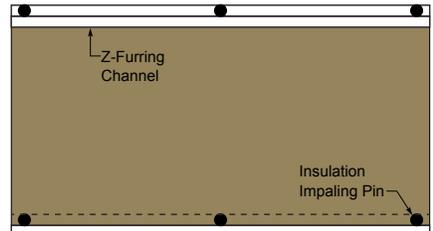
**Note:** For horizontal applications, utilize furring channels with integral drainage capacity measured per ASTM E2273.
