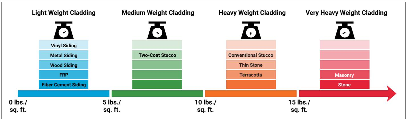
**Note:** Very heavy cladding materials, such as stone, should be evaluated on a project basis unless self-supporting.
